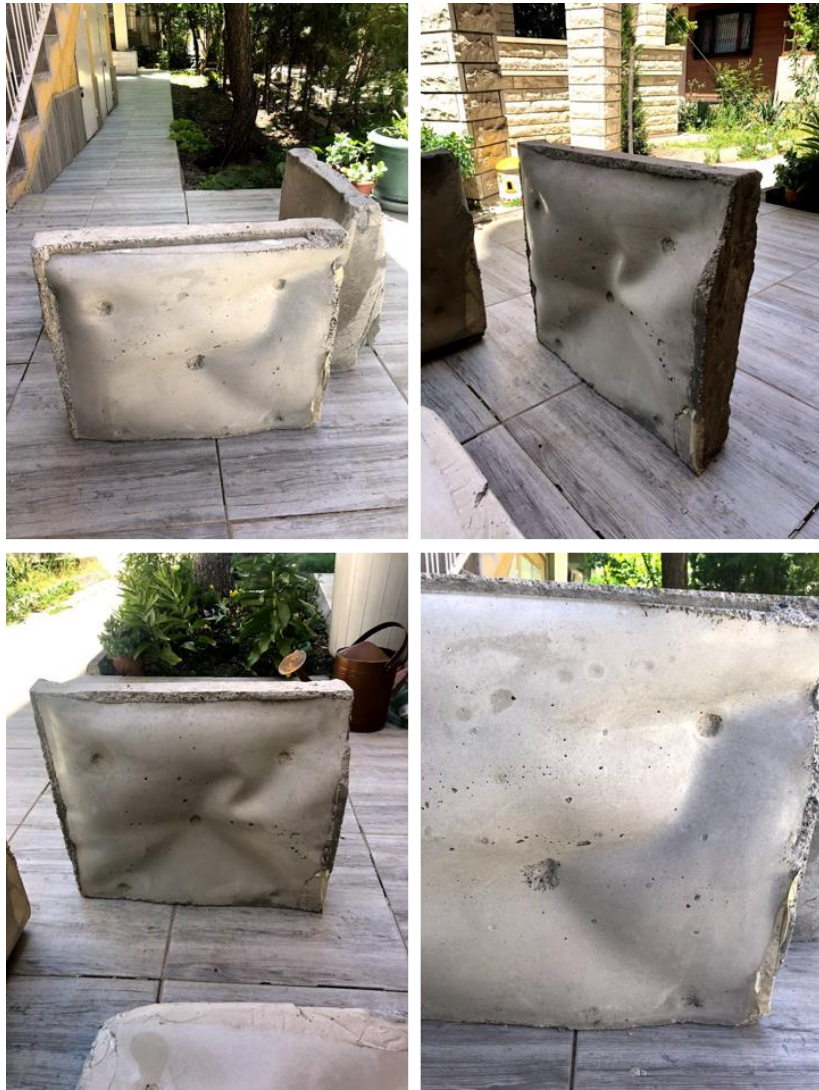
Figure 27: Second vertical concrete component production photographs, produced and photographed by the author
