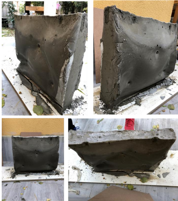
Figure 24: Vertical Concrete Component Production, first vertical concrete component production, produced and photographed by the author
