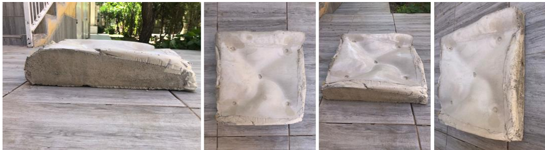
Figure 30: Horizontal concrete component production with adaptive and reusable tunnel formwork, produced and photographed by the author.
