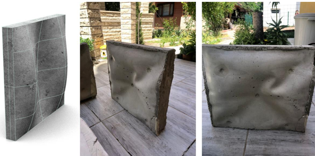
Figure 39: Designed component and produced concrete component differences. Designed mass created with vertical curves, so the form directly indicates the vertical curvature feature. (Produced and photographed by the author.)
