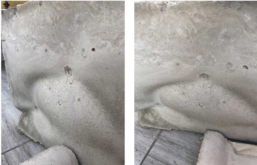
Figure 38: When surface material has insufficient tension and strain, it shows stretching due to pressure. (Produced and photographed by the author)
