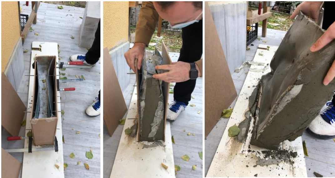
Figure 23: Concrete and formwork separation. Surface and concrete are easily separated without any break or shape deformation, produced, and developed by the author.
