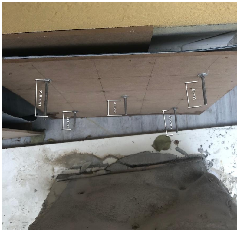
Figure 22: Pin distances are shown. These values match the vertical concrete production I / Side A, developed and photographed by the author.
