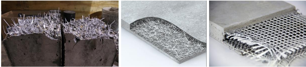
Figure 8: Fiber reinforcement methods with concrete.
